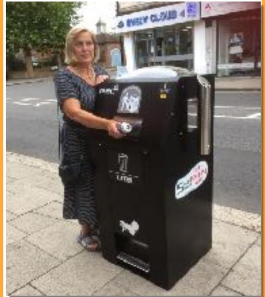
When waste in the bin reaches a set level, it is compacted using the power generated by the solar cells on the top of the bin. This allows more waste to be inserted, meaning the bins will not need to be emptied as frequently as a standard bin.
